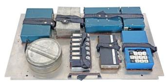
WSA 1 transmitter and associated equipment of system 32210 included an unknown high speed keyer (bottom right), which could be substituted by keyer 32843.
